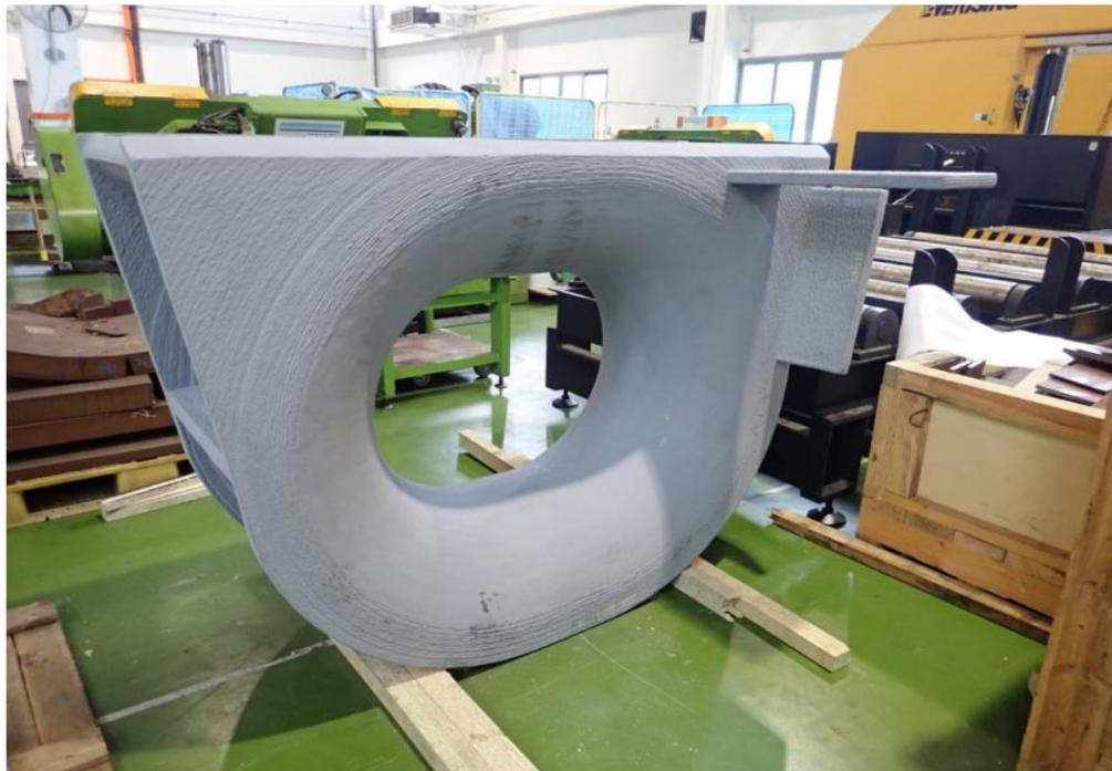
*Deck mounted type Panama Chock (SWL150Ton) produced during the additive manufacturing project.*
