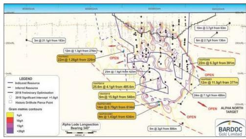
Figure 13: Alpha lode long section looking west, showing 2018 drilling, resource outline and optimised pit
