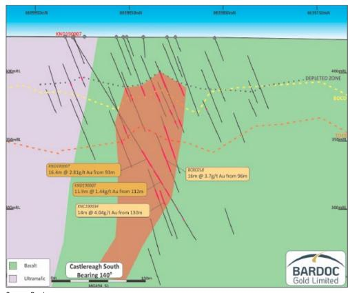
Figure 9: South Castlereagh composite cross section, looking north
