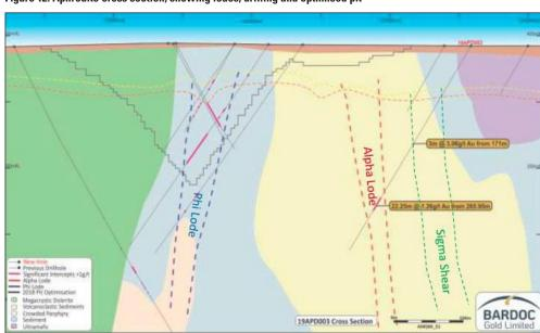
Figure 12: Aphrodite cross section, showing lodes, drilling and optimised pit
