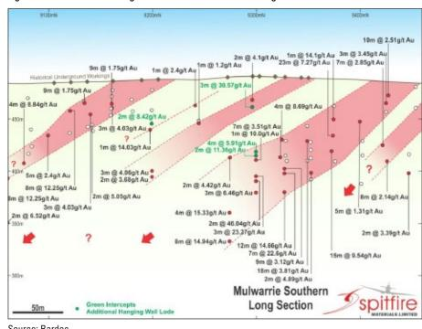
Figure 19: Mulwarrie South long section - doesn't show 2019 drilling
